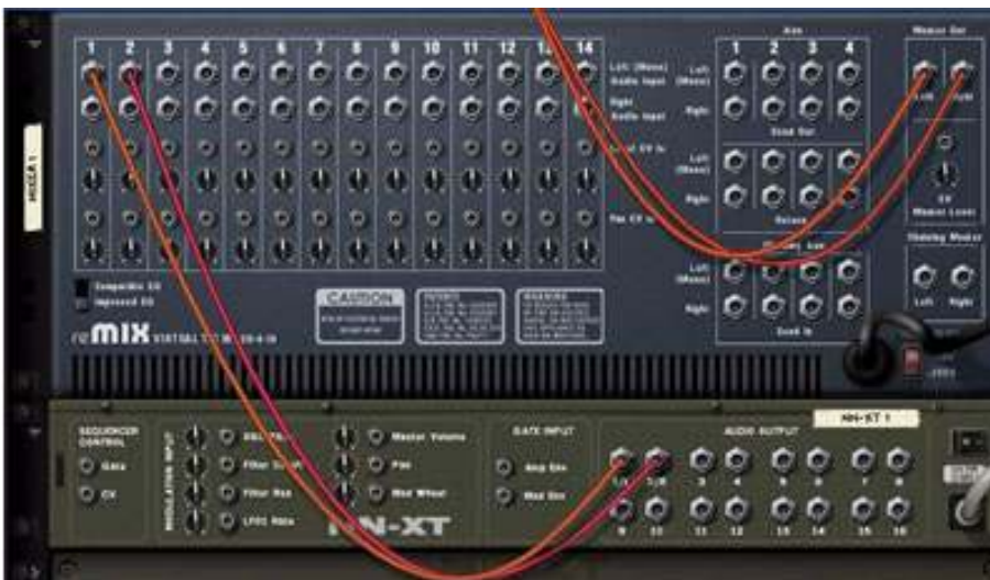
Fig 1: Sending the left and right output to separate channels.
